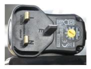
Set the voltage by turning the yellow selector on the inside of the power unit to 6 and plug in to the mains. Increase the voltage until you feel vibration throughout the instrument. \*Settings 6 or 7.5 for violin and perhaps higher for cello or bass seem good compromises between strength of vibration and quiet running. The unit is quite safe up to the
