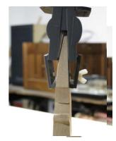
provide a positive mechanical connection between the adapter and the wooden bridge, enhancing the transmission of vibrations whilst minimising noise.
