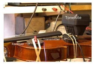
A separate ToneRite is needed for each instrument.
