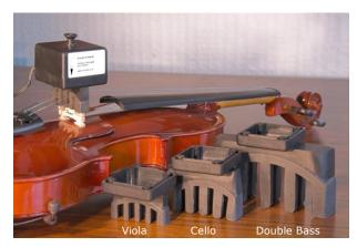
In the Mk 2 version, base plates are available for violin, viola, cello and double bass (see left), and fit to the vibrator by four screws. One vibrator and four base plates thus cover the whole string family. Also, the minimum operating frequency (and noise) is lower than that of the Mk 1.
