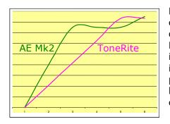
Readings were also taken to assess the "acoustic conductance" of the violin when stimulated by both devices rather than by specific notes of the AE Mk3. Starting with virgin instruments in both cases, it is clear that both devices caused an improvement in response over the 6 days (see left). The AE Mk2 peaks at 3 days whereas the ToneRite takes 2 days longer. This is probably due to the relative powers of vibration of the two devices.
